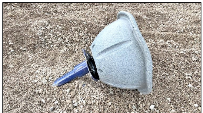
Tilted spinner seat damaged during turf installation
